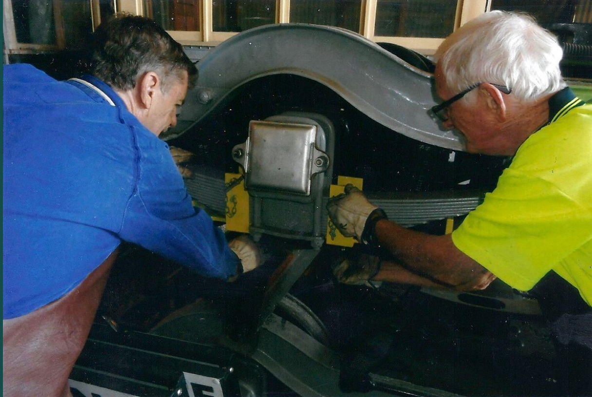
Two members fitting a member's designed leaf spring holder to a No. 15 truck.
