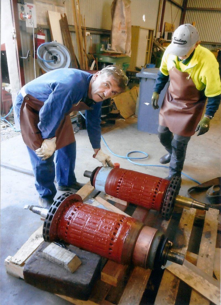
(Above) – Society members carrying out maintenance with two refurbished armatures from Met Vic 101 motors, a motor to axle gear casing being painted with undercoat, and checking a bogie bolster ready to go into a No. 15 frame.
