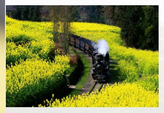
Now on the track, six steam locomotives still remain in working condition. Typed as ZM16-4 they were built by the Shijiazhuang Motive Power Machinery Works in the 1950s and 1960s as coal-burning locomotives with 0-8-0 wheel arrangement on narrow-gauge track, weighing 16 tons, delivering 3,168kg tractive effort, generating 1.3MPa working pressure from the boiler and running at a maximum speed of 35km/hour with a control speed with passengers at 20km/hour.
